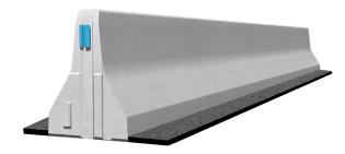
The vehicle restraint system 84XEA.3\_8 is embedded 40mm in asphalt or concrete and is mainly used, where a high containment level is needed within a narrow space.
